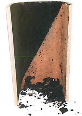
Creosote falls off easily as PCR dries
